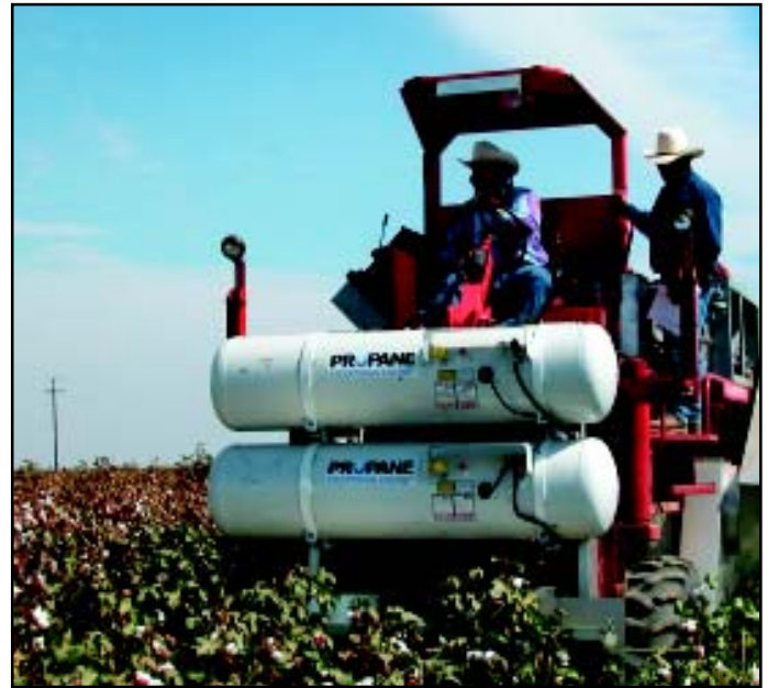
An experimental propane thermal defoliator is one of many projects you support through NPGA or PERC.
